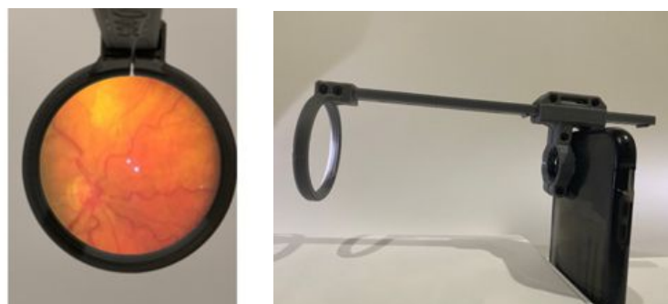
Figure 5. The left image shows the device camera view from a retinal fundus image (device tested on and image taken from real retina, background replaced with white). The right image shows the 3D-printed device fitted to the smartphone, which is the device configuration (lens was removed).
