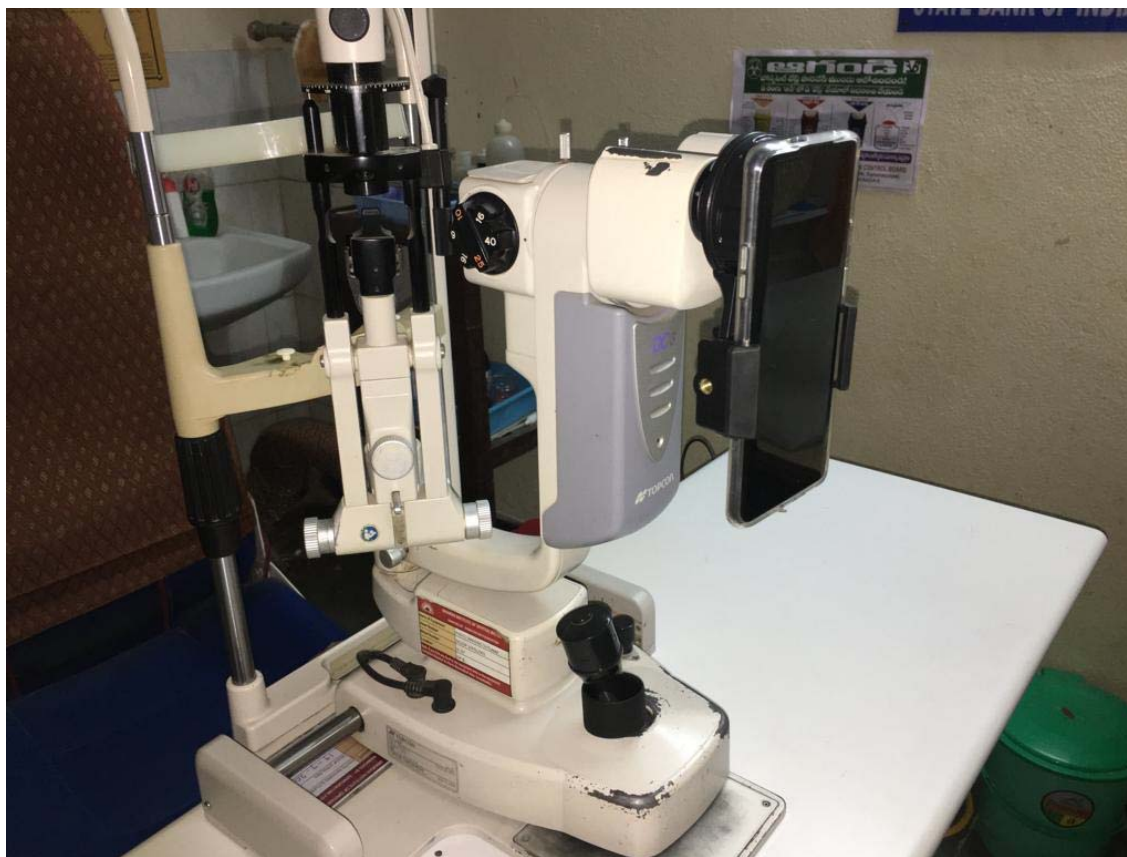
Figure 1: Imaging Setup of Smartphone-based Method. OnePlus 7 Pro smartphone is shown attached to Topcon slit lamp.
