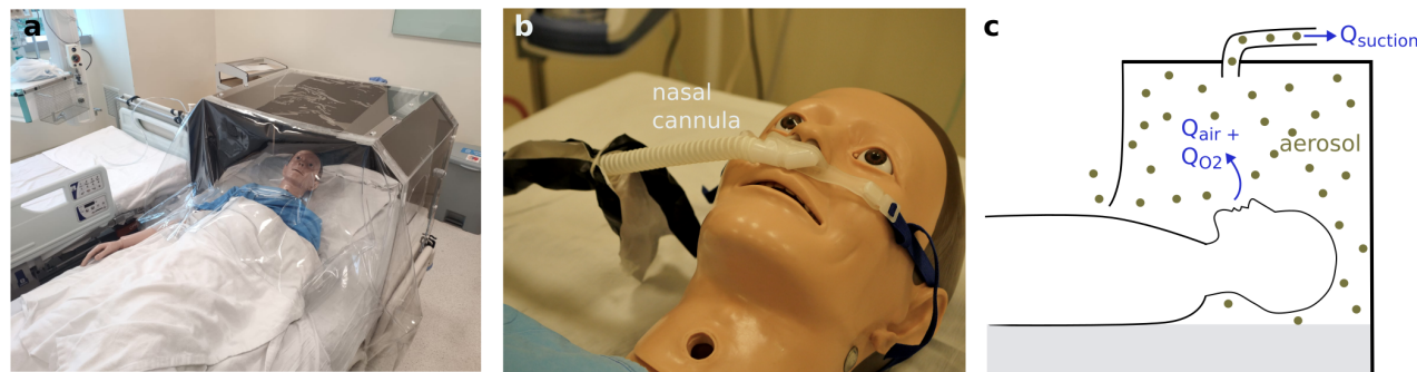
FIG. 1. (a) Barrier enclosure used to contain aerosols from patients who typically require supplementary oxygen treatment (b) delivered through a nasal cannula. (c) For effective containment of aerosol (gray dots), the suction rate Q_{\text{suction}} must be higher than the oxygen flow rate Q_{\text{O}_2} and the breathing (expiration) rate of the patient Q_{\text{air}} combined.
