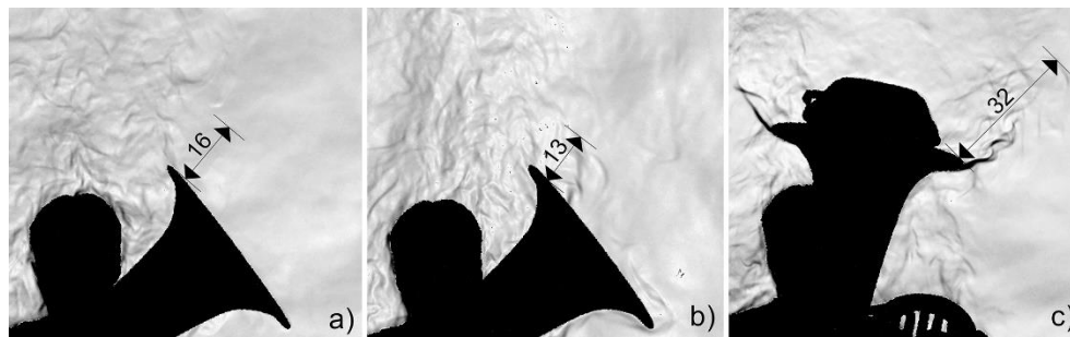
Fig. 22 Maximal range of the air escaping from the bell of the F tuba while playing the note F1 \approx 44 \text{ Hz} (a), note F4 \approx 349 \text{ Hz} (b), and with damper (c) [cm]
