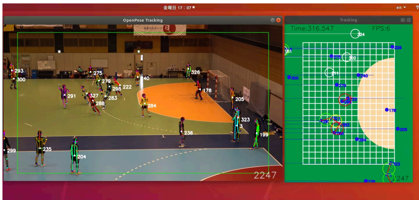
Figure-1: Real-time automated quantitative monitoring of social distancing with motion image-based AI system, shown on Ubuntu 18.04.5 LST. This system identified the participant positions using a function on OpenPose (17). The distance between the players was calibrated based on known court geometry. Once the system identified a pair of athletes within 2m, a white circle appears on the right window. Each additional second, the color of circle turned: green (2 seconds), yellow (3 seconds) and red (>4 seconds).
