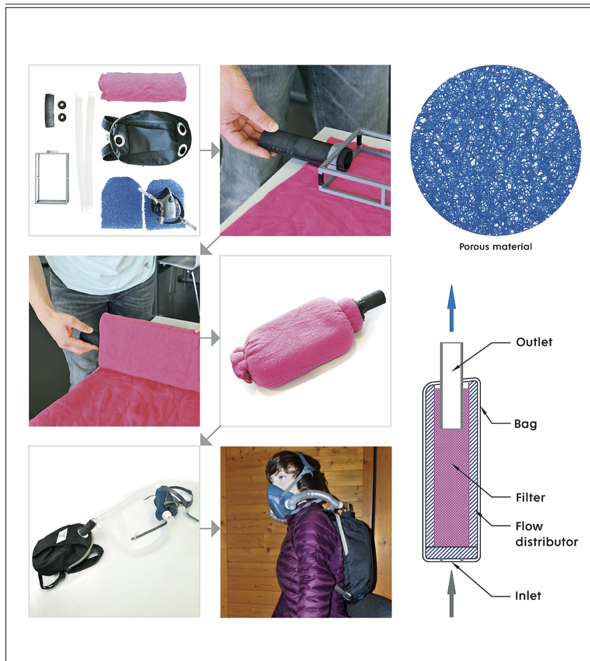
228 229 Fig 3. Assembly scheme of the filter kit. 230 Shown are all parts of the filter kit and its gradual assembly, including a demonstration of how it is to 231 be worn (manikin). The purpose of the blue porous material is to allow air to access the filter cartridge;
