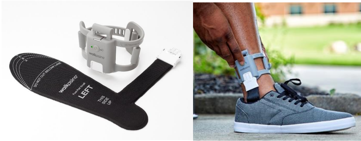
Figure 1. (Left) The two components of the Walkasins device, the pressure sensitive flexible foot pad that is placed in the shoe and connects to the leg unit that contains a rechargeable battery, a microprocessor, supporting electronics, and four tactile stimulators. The embedded software algorithm evaluates pressure data and activates tactile stimulators at relevant times during standing and walking to signal balance-related information to the afferent nervous system. (Right) A Walkasins user wearing the device in the process of turning it on. The Walkasins system is worn bilaterally (unilateral components depicted).
