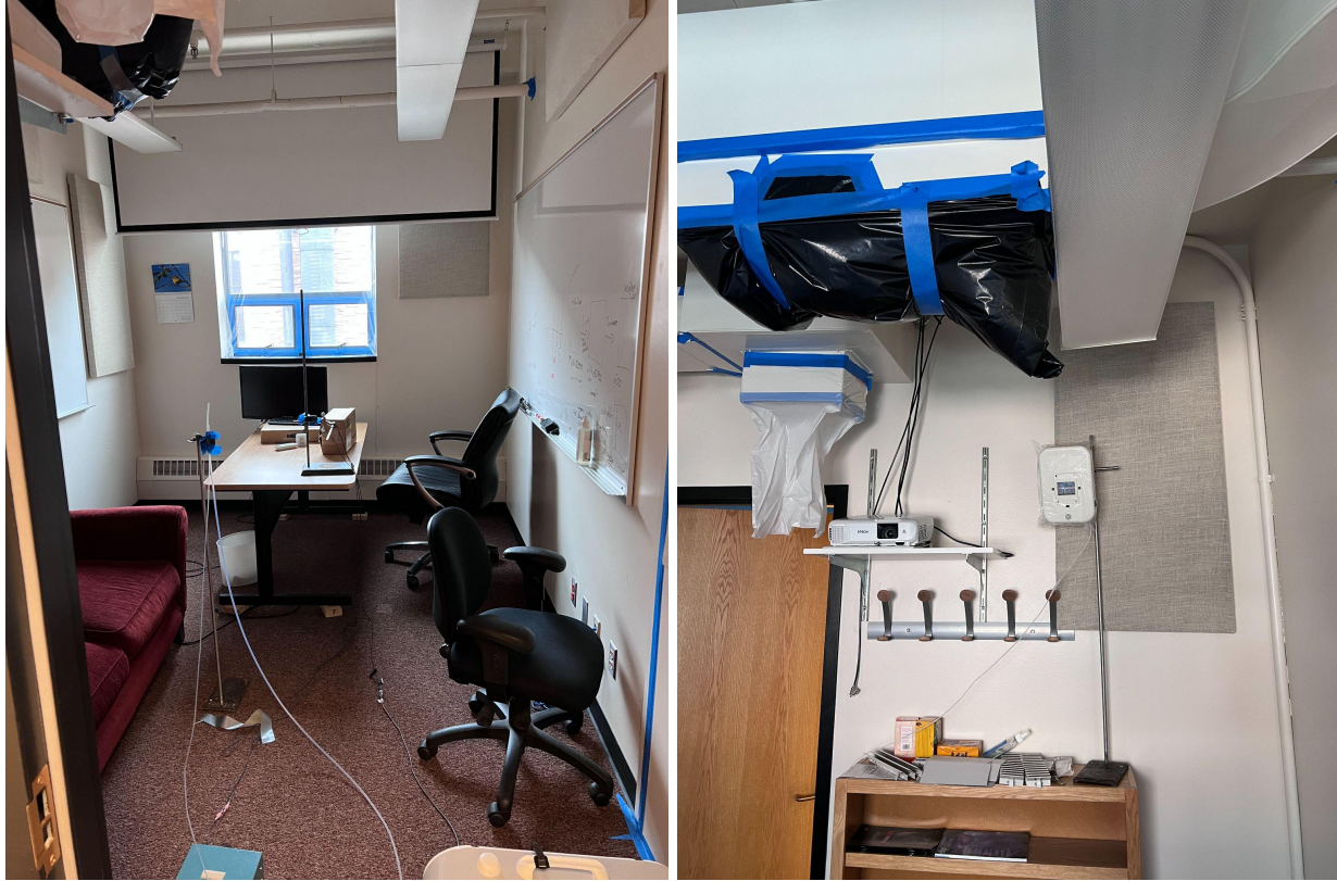
Figure S3. Experimental setup in the test office. The O_3 sampling tube and CO_2 injection tube were placed in the middle of the room on a ring stand (left). The GUV lamp was placed high in the room against the West wall of the room (right). The path of the light was interrupted by the furniture and walls, and the effective pathlength in the main paper was estimated to account for those obstructions.
