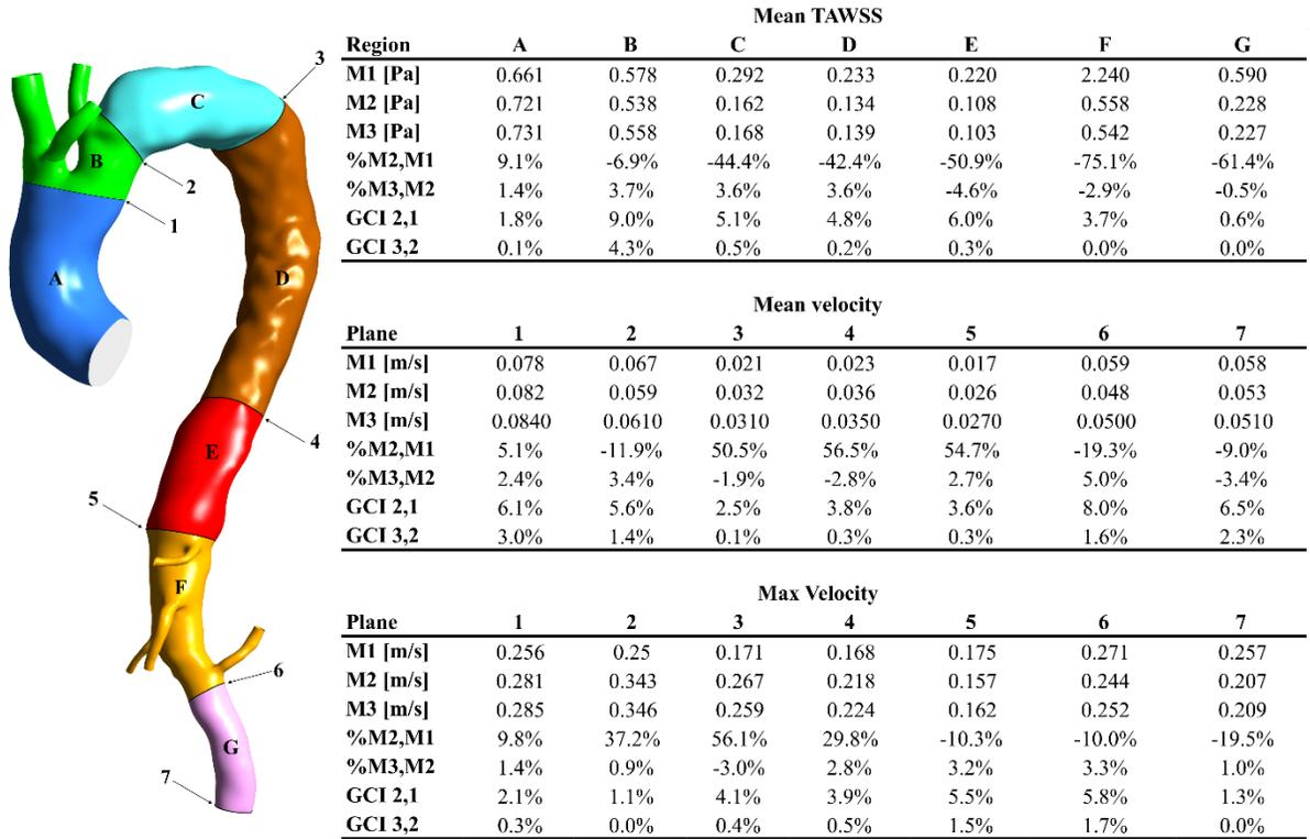
**Figure 1:** On the left side are planes and regions of interest, denoted by numbers and capital letters. On the right side, tables display the relative error and GCI comparison for M1, M2, and M3 regarding the mean TAWSS and mean and maximum velocity.
