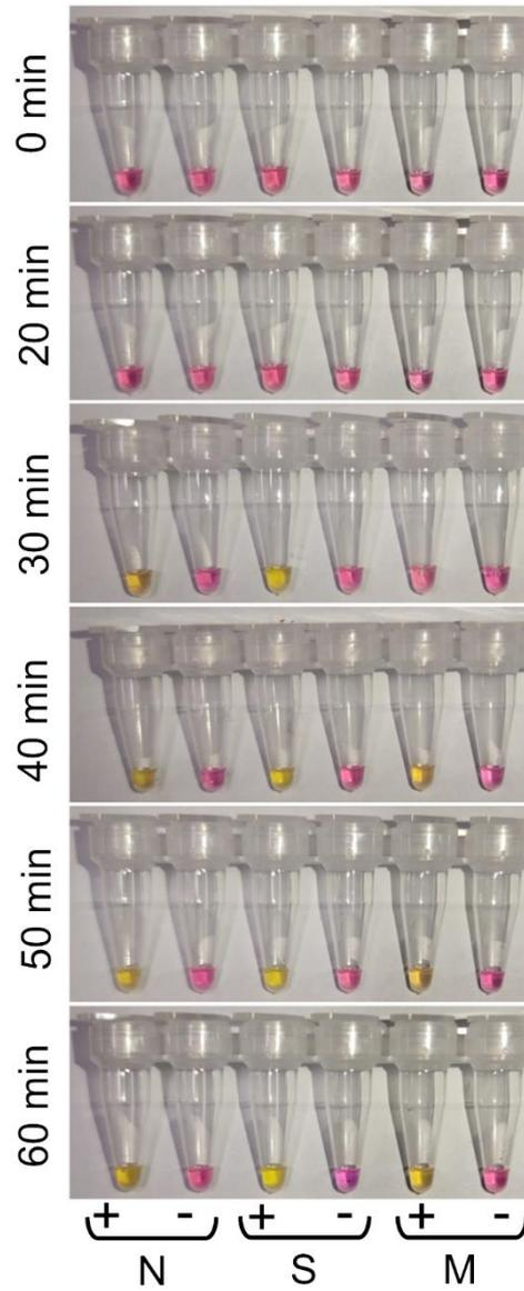
**Fig. S4:** Optimization of reaction time was performed at 65°C temperature on the basis of three set gene specific primer (N, S and M). Typical yellow color changes of all sets were observed within 40 min. N: Nucleocapsid gene, S: Spike gene, M: Membrane protein gene
