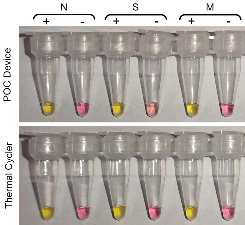
**Fig. S7:** RT-LAMP reaction performed in in our detector and thermal cycler to check the present test performance as compared to that using a thermal cycler. N: Nucleocapsid gene, S: Spike gene, M: Membrane protein gene
