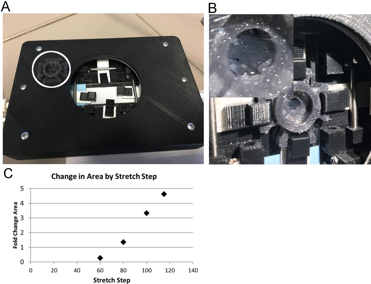
Figure 5: 3D-printed Confocal Microscope Lung Stretching Device. (A) Four motors are housed within a plastic case that fits within the microscope mounting plate. A silicone mold (circle) is secured by four clips attached to the motors by Tyvek strips. (B) Image of lung before stretching and after stretching (inset). (C) Quantification of the increase in mold aperture area with number of stretch (steps). The steps used for imaging are shown.
