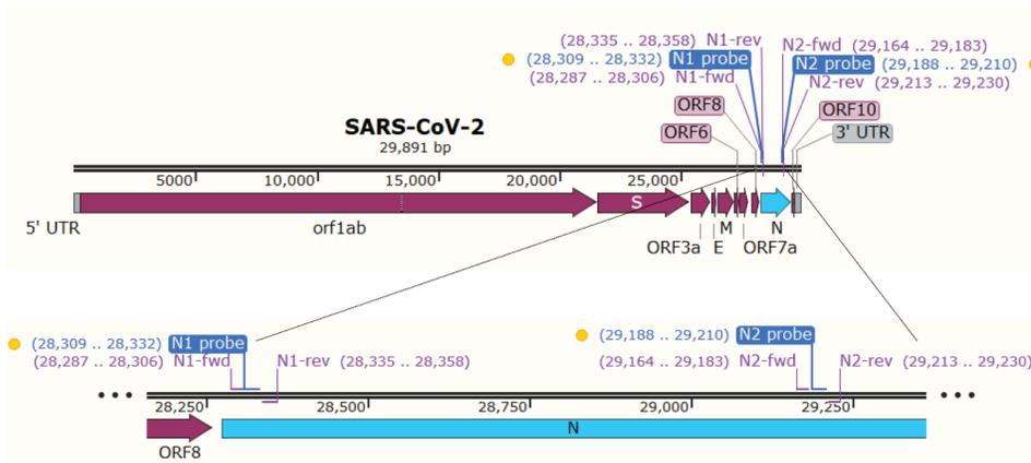
**Figure S1. Fluidigm chip layout and N gene probes.** (A) The 192x24 Fluidigm chip can analyze 192 samples (from two 96-well microtiter plates) against 24 assays. In our experimental design, each sample was analyzed with 9 replicates each of the N1 and N2 (viral N gene) assays and 6 replicates of the RP (human gene) assay. (B) Schematics showing the locations of the PCR primers and Taqman probes for the N1 and N2 assays on the SARS-CoV-2 genome.
